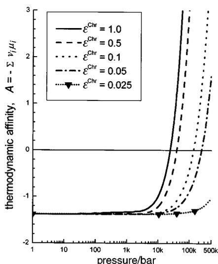
Fig. 4 The thermodynamic affinity,  $A(p, T; \alpha)$  of a chiral hard-body system of asphericity  $\alpha = 1.5$  and prolateness  $\beta = 2.25$  as a function of pressure for different values of the parameter of chirality,  $\varepsilon^{\text{Chr}}$ .
